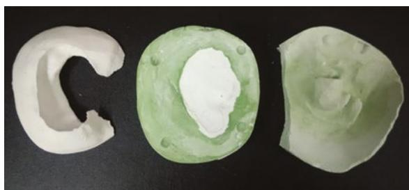
Fig. 7. 3-piece mould to process the silicone
